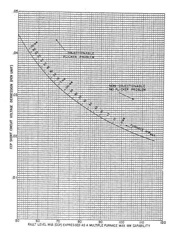
Fault level/MW  $_{\rm MAX}$  ratios and accompanying short circuit voltage depression.
